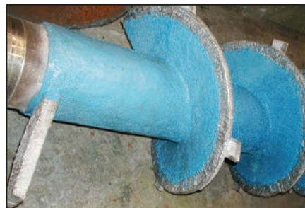
ARC MX1 applied and tips welded.
