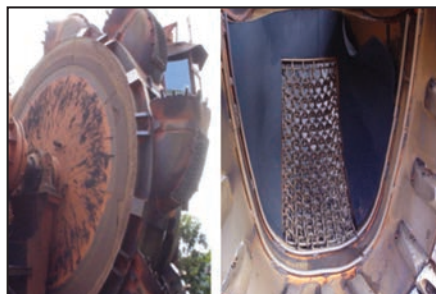
Repair life of 6 months with hard face welding.
