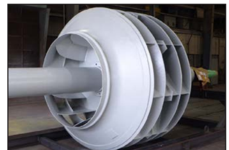
Dynamically balanced ARC S7 AR coated fan.
