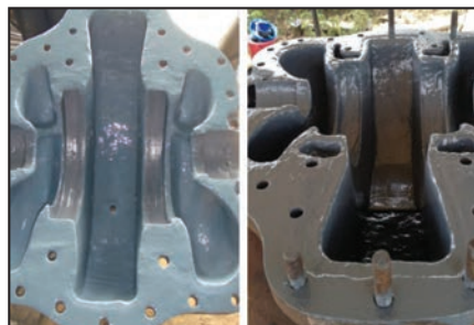
Repair being performed, body and cover.
