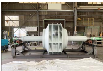
ID Fan in paint shop.
