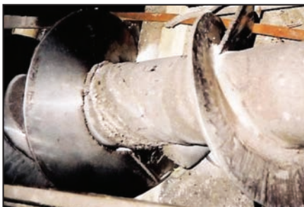
Abraded screw conveyor.
