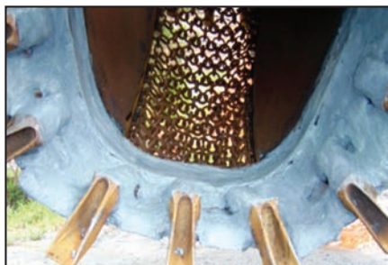
ARC BX1 coating applied to the borders between the teeth.
